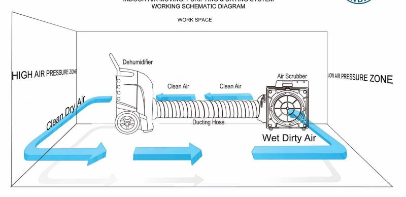
XPOWER's XD-125 is part of a revolutionary new Air Purification & Drying System which uses the combined power of the Air Scrubber and Dehumidifier to remove moisture and contaminants from the air!
